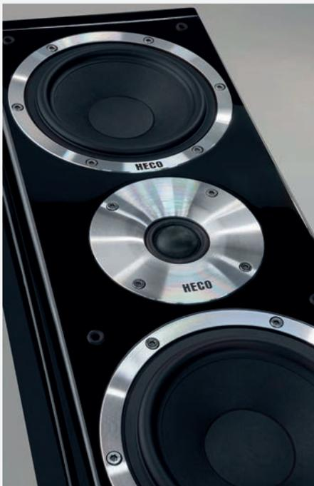
Heco's speakers also look good underneath their elegant facade: wooden elements inside the housing reinforce the most important sections of the speaker, while solid 25 mm thick MDF has been used for the front panel. The rather dainty 402 unit features a 2.5-way configuration. Two similarly constructed 13 cm chassis cater for the bass-midrange
